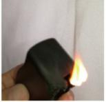
The material is not antiflaming, will not die after fire, is very dangerous 材料为非阻燃料,着火后不会熄灭,容易引起火灾,存在重大安全隐患。
