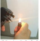
The material is antiflaming, will die automatically after fire 材料为阻燃料,着火后会自灭
