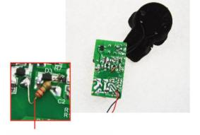
The resistance easy to catch a short circuit, and catch fire 此电阻容易引起短路,容易导致电源发热引起火灾
